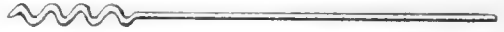
A tool with screw for pulling wires through small holes in insulation or walls
